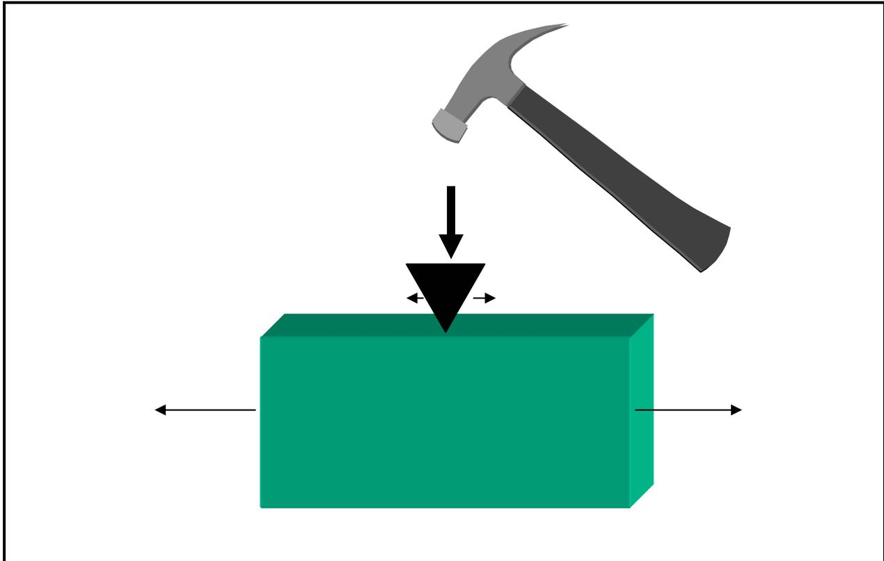
A knife cutting butter functions in the same way. You push downward on the top of the butter with a knife. The butter is not crushed under the edge of the knife, it is pushed apart into two pieces as the knife moves through it.
