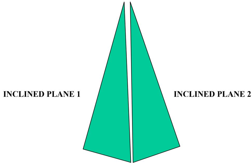
An inclined plane allows you to push a heavy load upward, parallel to the plane of the inclined board with less force than you would need to lift the object straight up.
