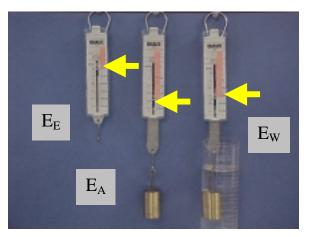
When the mass is in the water, the water pushes up on the mass, so the mass exerts less force on the spring scale and the spring scale is extended less. How much less force does the mass exert?
